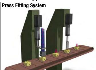
Force control is utilized to limit output force of actuator to press parts together. Similar applications include:
