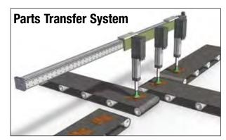
Network communication is utilized to control multiple actuators.
