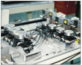
These Tol-O-Matic rack and pinion rotary actuators have run over 10,000,000 cycles carrying over the maximum rated loads for their bore size without fail.
