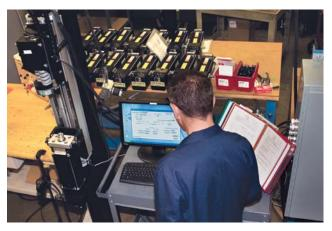
Functional unit testing for hundreds of cycles quantifies stroke, length, torque under no load, input current vs force standard deviation.
