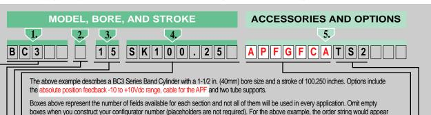
First, determine the model, the bore size and the stroke required.
