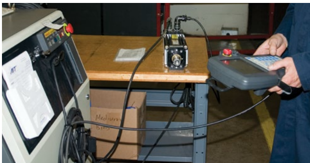
Final system test ensures the feedback device is properly aligned with the GSWA motor poles.
