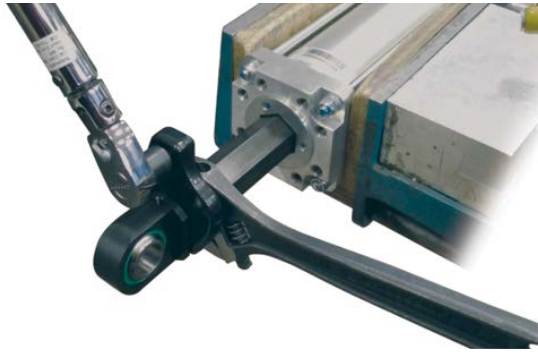
Figure 4.4: For Hex rod, hold thrust rod stationary using a wrench on the flat of the rod when attaching accessories, linkages or load to the actuator. Use a torque wrench to tighten the interfacing rod end to the actuator threaded connection point. Torque values provided in Table 4.1
