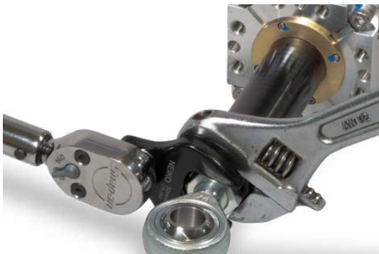
Figure 4.3: Hold thrust rod stationary using a wrench on the flats of the rod end when attaching accessories, linkages or load to the actuator. Two wrenches are used here: The silver wrench prevents the thrust rod from rotating, the blue wrench will fasten the spherical rod eye option to the actuator rod end.
