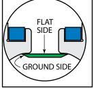
Insert Sealing Band (19) into Cylinder Tube (26) by laying the Band out along the length of the actuator and passing it sideways through the slot in Tube. With flat side facing up (ground side facing down), position the Band so the length of band sticking out the end of the Tube is as long as Piston Assembly. (5 - 10 inches or 12 - 25 cm)
