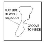
the Pistons (2) into the Piston Bracket (1), with Band Ramp up, until Piston Bracket (1), with Band Ramp up, until Piston snaps into hole in Piston Bracket. Install new lubricated U-Cups (3) (seal lips facing out), and Cushion Seals (4) (small end facing out). Slide new Wipers (7) into the groove on the Piston Bracket (1) until flush with end. Trim off excess flush to other end of Piston Bracket. Wipers need to be installed with the flare edges facing outward.
