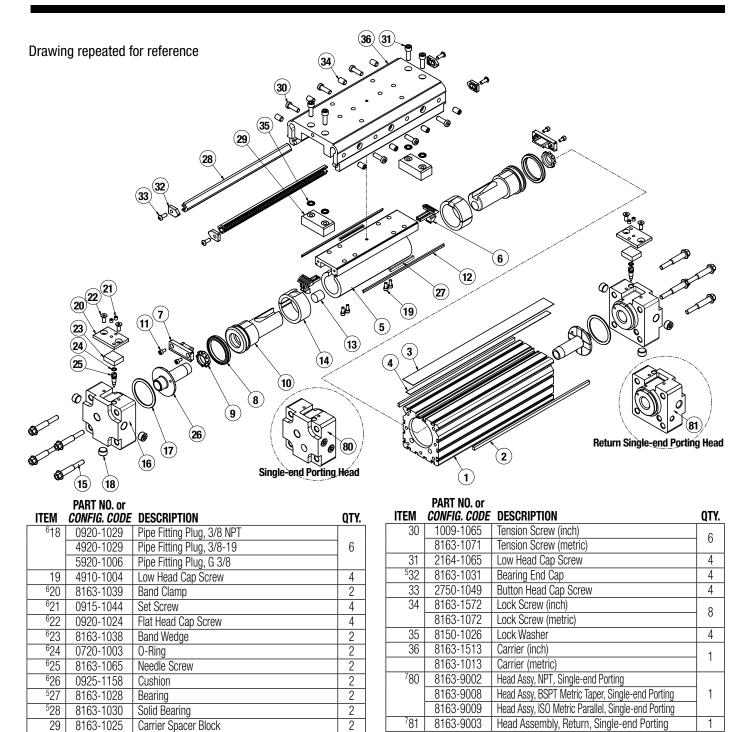
Auxiliary Carrier Option Note: If replacing a Tube (1.), Magnet Band (2.), Dust Band (3.), or Seal Band (4.) on an actuator that has an Auxiliary Carrier, be sure to add "DW\_\_\_\_" to the end of the configuration string when ordering. "DW" indicates the need for additional length and "\_\_\_" indicates the measurement of space between carriers (in inches [SK] or millimeters [SM] as indicated earlier in the configuration string).
