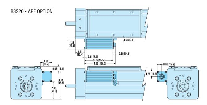
Unless otherwise noted, all dimensions are in inches [dimensions in brackets are in millimeters]
