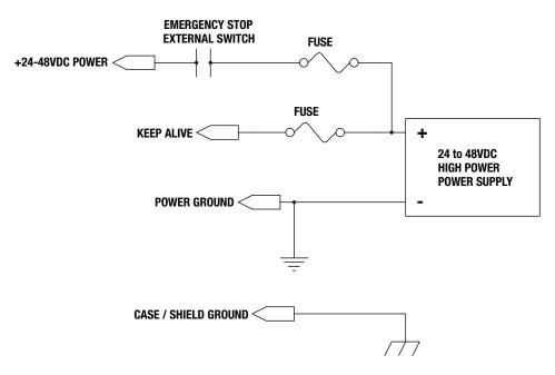
Figure 2-15: ICR SV1B Basic Actuator Single Supply - External Cut-off Switch for Emergency Stop
