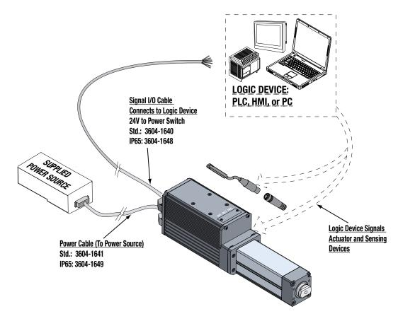
Figure 2-16: ICR SV1B Basic Actuator Setup
