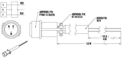
Figure 2-2: ICR SV1B Basic Actuator IP65 Power Cable 3604-1649
