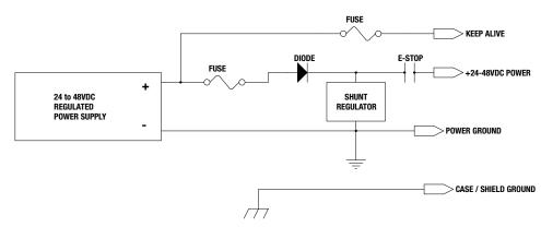
Figure 4-4: Regulated Power Supply with Blocking Diode and Shunt Regulator
