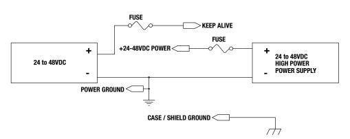
Figure 2-13: ICR SV1B Basic Actuator Logic and Main Power Supplies
