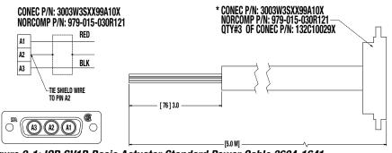
Figure 2-1: ICR SV1B Basic Actuator Standard Power Cable 3604-1641
