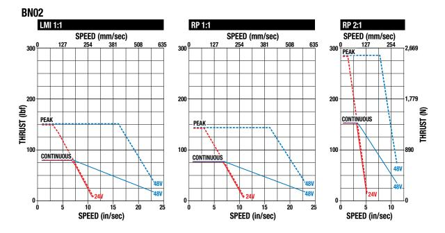
Figure 1-2: BN02 Ball Nut: Continuous and Peak Speed vs Thrust
