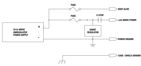
Figure 4-2: Unregulated Power Supply Configuration with Shunt Regulator
