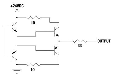
Figure 2-11: ICR SV1B Basic Actuator Output Interface Circuit Diagram
