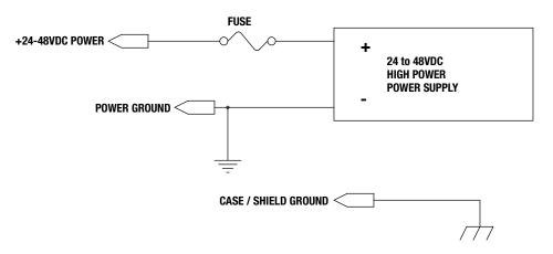
Figure 2-14: ICR SV1B Basic Actuator Single Supply - Main Power
