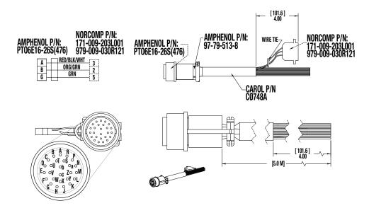
Figure 3-4: ICR/ICM SV1P Plus IP65 I/O Cable 3604-1648
