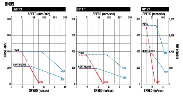
Figure 1-1: BN05 Ball Nut: Continuous and Peak Speed vs Thrust
