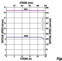
Figure 1-4: ICR SystemCritical Speed
