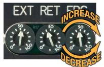
Figure 5-8: ICR SV1B Basic Actuator Force Control Potentiometer
