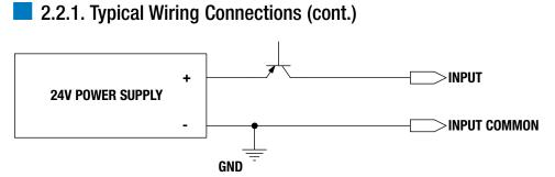
Figure 2-8: ICR SV1B Basic Actuator Input Source (PNP) Connection
