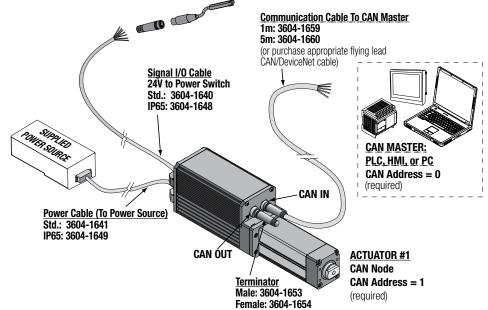
Figure 3-21: ICR/ICM SV1P Plus Single Actuator Setup for optional CANopen Position Control
