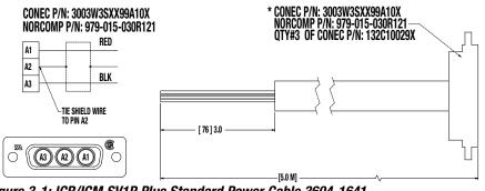
Figure 3-1: ICR/ICM SV1P Plus Standard Power Cable 3604-1641
