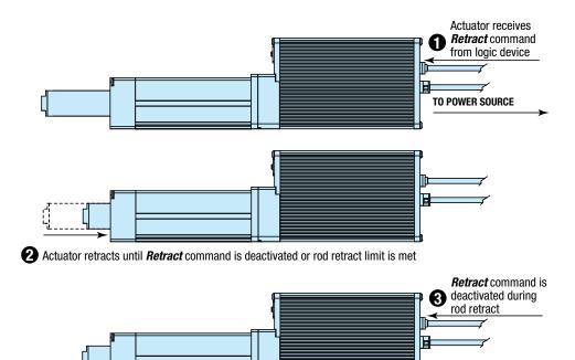
Actuator decelerates to stop and holds position
