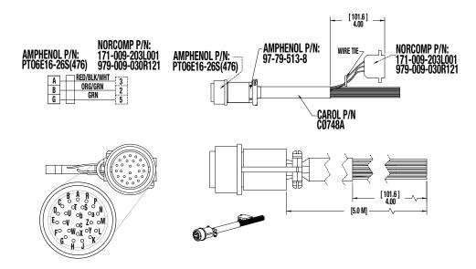
Figure 2-4: ICR SV1B Basic Actuator IP65 I/O Cable 3604-1648
