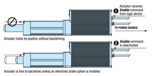
Figure 5-1: ICR SV1B Basic Actuator Enable Input Command
