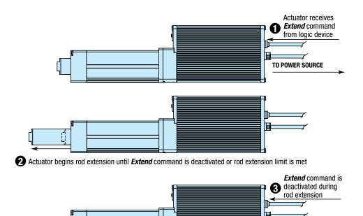
Actuator decelerates to stop and holds position
