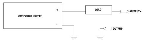
Figure 3-15: ICR/ICM SV1P Plus Digital Output Sinking Wiring Diagram
