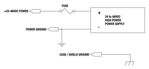
Figure 3-18: ICR/ICM SV1P Plus Single Supply - Main Power
