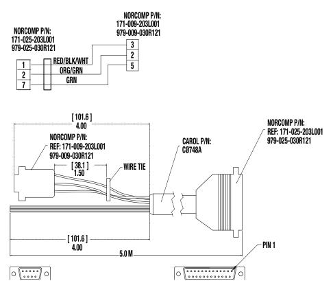
Figure 3-3: ICR/ICM SV1P Plus Standard I/O Cable 3604-1640
