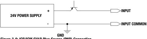
Figure 3-9: ICR/ICM SV1P Plus Source (PNP) Connection
