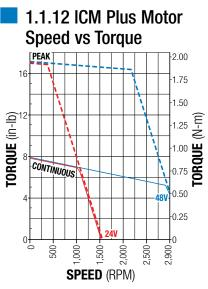
Figure 1-5: ICM Plus Motor Speed vs Torque
