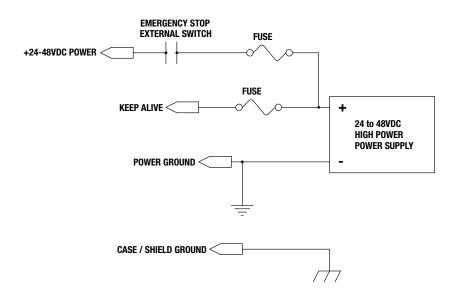
Figure 3-19: ICR/ICM SV1P Plus Single Supply - External Cutoff Switch for Emergency Stop
