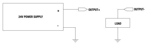
Figure 3-16: ICR/ICM SV1P Plus Digital Output Sourcing Wiring Diagram
