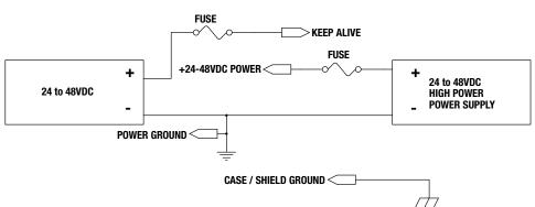
Figure 3-17: ICR/ICM SV1P Plus Logic and Main Power Supplies
