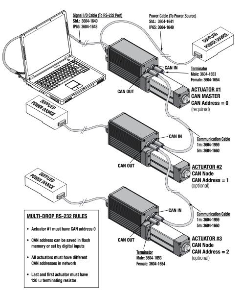
Figure 3-22: ICR/ICM SV1P Plus Multi-drop RS-232 Setup (RS-232 to optional CANopen)
