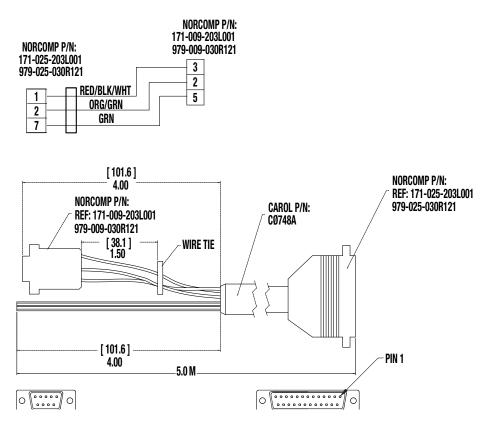
Figure 2-3: ICR SV1B Basic Actuator Standard I/O Cable 3604-1640
