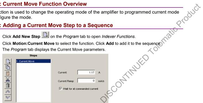
Choose appropriate values for the following parameters. Enter numeric values directly or enter the number (R0-R31) of an Indexer 2 Program register. See Using Registers to Pass Values to Functions (p. 38).
