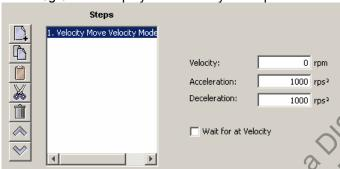
■ Choose appropriate values for the following parameters. Enter numeric values directly or enter the number (R0-R31) of an Indexer 2 Program register. See Using Registers to Pass Values to Functions (p. 38).
