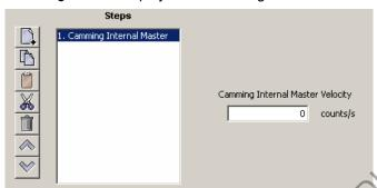
Choose appropriate values for the following parameter. Enter the velocity directly or enter the number (R0-R31) of an Indexer 2 Program register. See Using Registers to Pass Values to Functions (p. 38).
