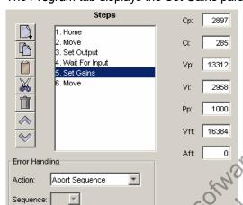
Choose appropriate values for the following parameters. Enter number values directly or enter the number (R0-R31) of an Indexer 2 Program register. See Using Registers to Pass Values to Functions (p. 38).
