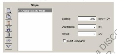
■ Choose appropriate values for the following parameters. Enter numeric values directly or enter the number (R0-R31) of an Indexer 2 Program register. See Using Registers to Pass Values to Functions (p. 38).
