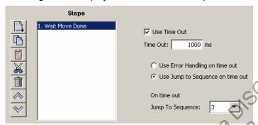
Choose appropriate values for the following parameters. Enter the *Time out* value directly or enter the number (R0-R31) of an Indexer 2 Program register. See Using Registers to Pass Values to Functions (p. 38).
