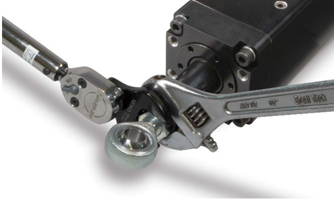
Figure 4.5: Hold thrust rod stationary using a wrench on the flats of the rod end when attaching accessories, linkages or load to the actuator. Two wrenches are used here: The crescent wrench prevents the thrust rod from rotating, the torque wrench will fasten the spherical rod eye option to the actuator rod end. Torque values provided in Table 4.1
