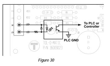
In some applications it may be advantageous to use a PLC or controller to monitor the drive's fault output for fault conditions. The diagram in Figure 30 illustrates the recommended circuit for connection to a PLC or logic controller.
