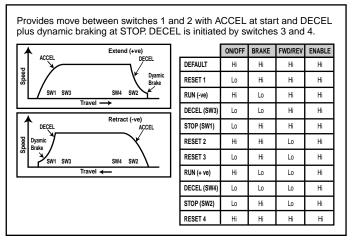
*Figure 39* The application illustrated in Figure 38 uses four normally open reed
