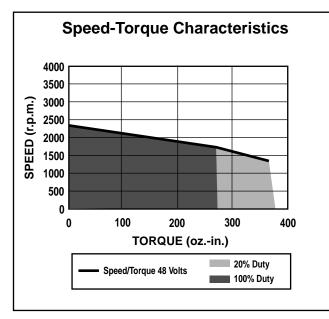
KE: 22.5 Volts/1000 r.p.m. KT: 30.5 oz.-in./Amp. Ra: 0.6 Ohms Rotor Inertia: 100.67 oz.in.2 Max. Temp.: 105° F. Weight: 17 Ibs.
