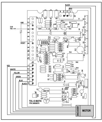
There are six wires connecting the Encoder to the Drive Module. Terminal connections are +5Vdc to power the encoder, encoder GND, and the other four are connected to the A and B channels, and serve as the encoder feedback to the dc closed loop drive module. Use of shielded cable is strongly recommended with the shield grounded at one end only
