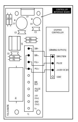
Instructions for connecting the DMCLDC drive to a "generic" stepper controller are provided below and are illustrated . The pulse and direction inputs to the drive are opto-isolated on the Controller Interface Board.
