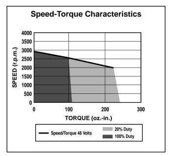
KE: 15.83 Volts/1000 r.p.m. KT: 20.35 oz.-in./Amp. Ra: 0.51 Ohms Rotor Inertia: 20.48 oz.in.2 105° F. Max. Temp.: Weight: 8.4 lbs.
