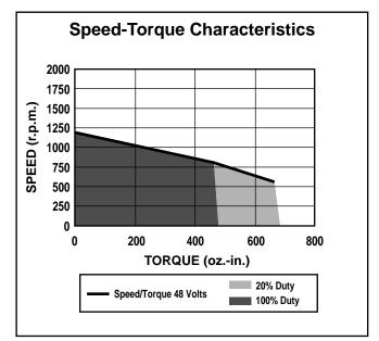
KE: 35.8 Volts/1000 r.p.m. KT: 48.4 oz.-in./Amp. Ra: 0.87 Ohms Rotor Inertia: 122.28 oz.in.2 Max. Temp.: 105° F. Weight: 20 Ibs.
