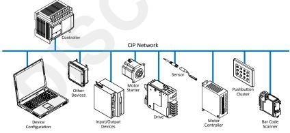
Figure 1-1: EtherNet/IP Network Example
