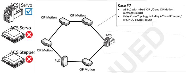
CASE #7: PLC sending CIP Motion messages in Rockwell device level ring (DLR) with ACSI motor/drive/controller
