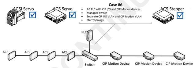
CASE #6: AB PLC with CIP I/O and CIP Motion devices through switch
