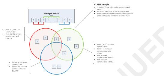
Figure 1-4: VLAN Diagram
