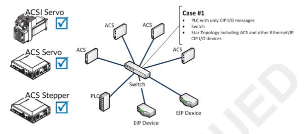
CASE #1: PLC with only CIP I/O messages -> switch -> star topology of ACS drives and other EtherNet/IP devices
