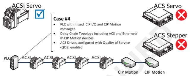
CASE #4: PLC with CIP I/O and CIP Motion messages  $\rightarrow$  daisy chain topology of ACS drives and other EtherNet/IP devices
