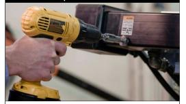
**WARNING** Set drill to low torque setting to prevent excessive torque from damaging Manual Override Tool or the GSWA
