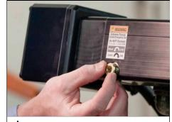
**WARNING** Manual Override Tool must be removed and Manual Override Access Plug replaced before powering GSWA
