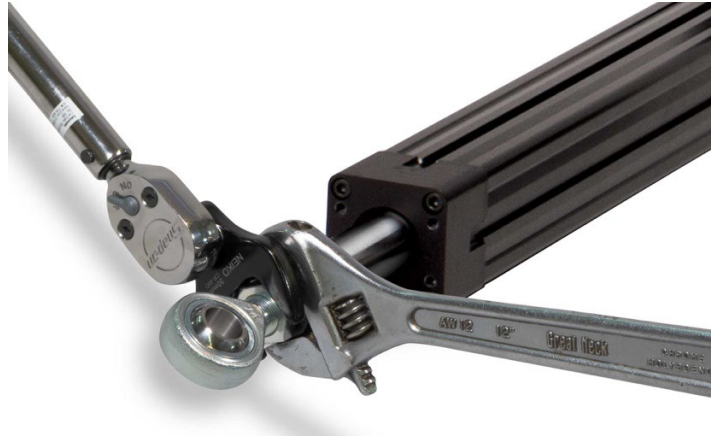
Figure 4.3: For RSA hold thrust rod stationary using a wrench on the flats at the end of the thrust rod when attaching accessories, linkages or load to the actuator.
