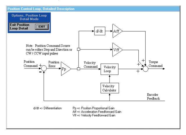
Figure 4.0: Block Diagram showing Positioning Mode Control Functions
