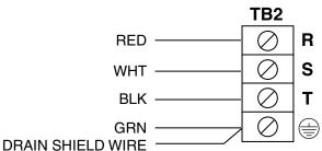
Figure 6.1 - DV10/20/30 Motor Power Cable Connections for MRV 2X, 3X, 5X
