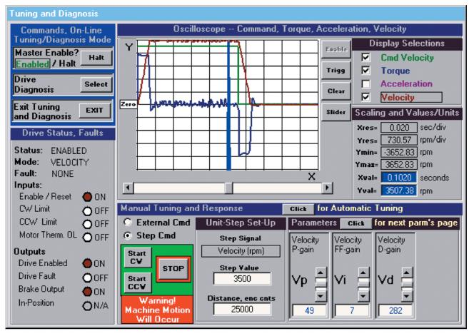
Figure 3.5: Velocity Step-Response after Manual Tuning Adjustments
