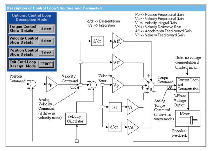
Figure 4.2: Block Diagram of All Drive Control Functions
