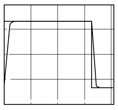
Figure 12.5 Critically Damped Signal (Ideal Tuning)
