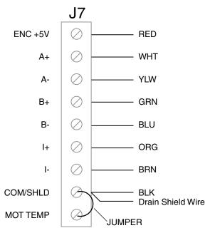
**NOTE:** Tol-O-Matic MRB brush servo motors do not include a thermal switch. Place wire jumper between COM/SHLD and MOT TEMP terminals. The drive's I<sup>2</sup>T motor protection is still active to provide motor overheating protection.
