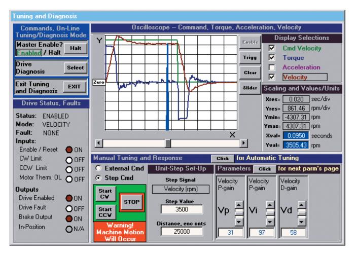
Figure 3.4: Velocity Step-Response after Auto-Tuning
