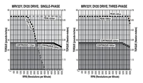
Figure C.10- MRV 33Y DV10/20 Single-Phase, Three-Phase Drive
