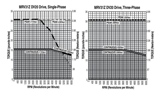
Figure C.7- MRV 31Z DV20 Single-Phase, Three-Phase Drive
