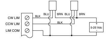
Figure 9.3 - Limit Switch Connections
