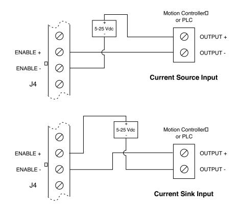
Figure 9.4 - Enable Input Connections
