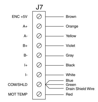
Figure 6.2 - DV10/20/30 Motor Encoder Connections
