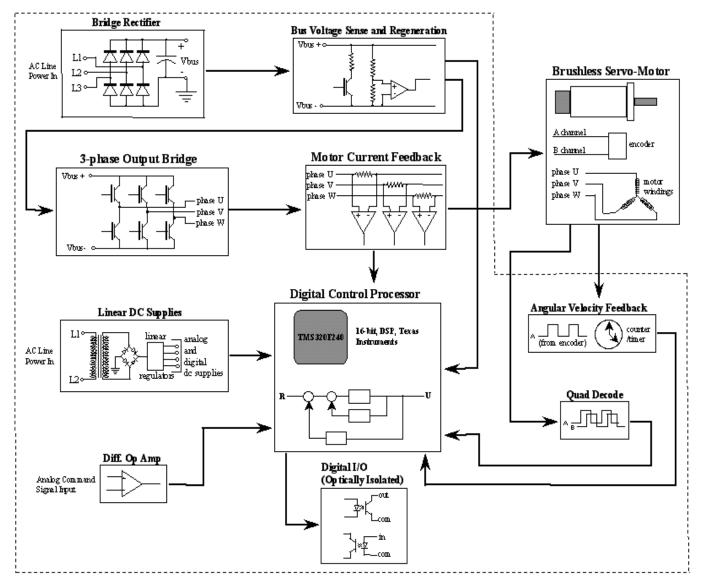
Figure 1.0: Diagram of Drive Hardware Functions
