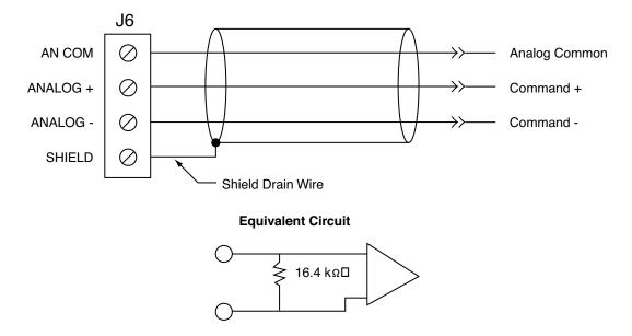
Figure 10.1b - Torque/Velocity Mode Connections (continued)
