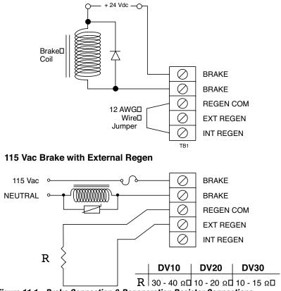
Figure 11.1 - Brake Connection & Regeneration Resistor Connections
