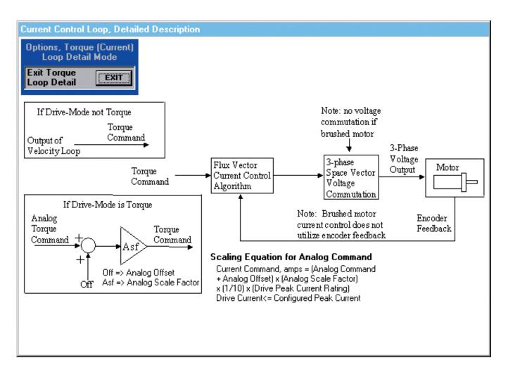
Figure 2.0: Block Diagram showing Torque-Mode Control Functions
