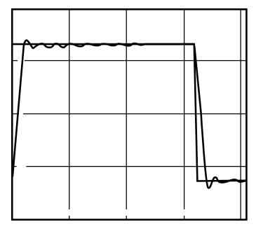
Figure 12.3 - Underdamped Signal
