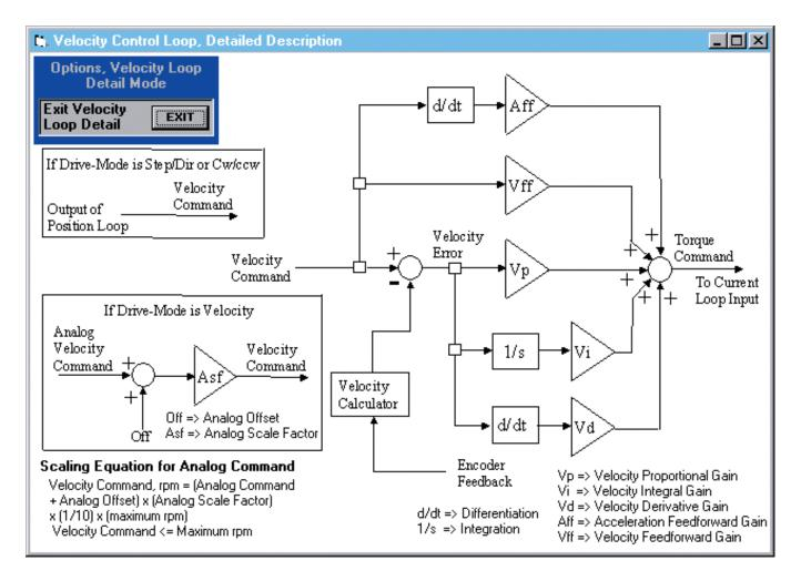
Figure 3.0: Block Diagram showing Velocity-Mode Control Functions
