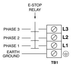
Figure 6.5 - Special E-Stop Connections
