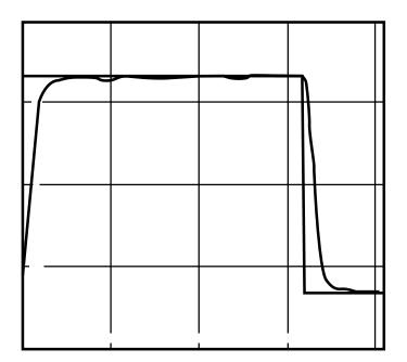
Figure 12.4 - Overdamped Signal
