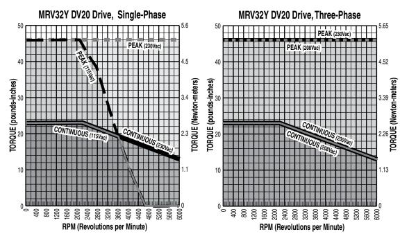
Figure C.8- MRV 32Y, DV20 Single-Phase, Three-Phase Drive
