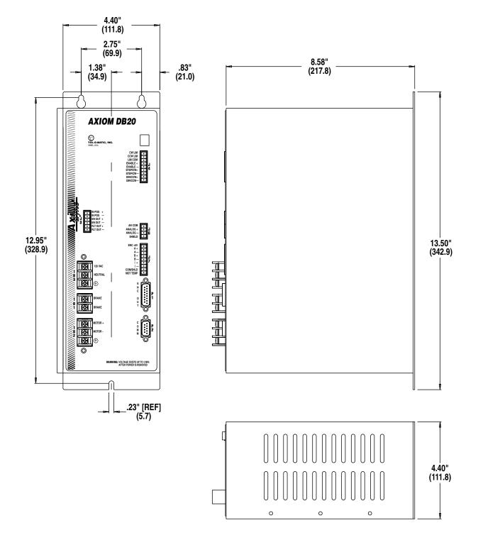
Figure 4.3 - Axiom DB20 Drive Mounting Dimensions
