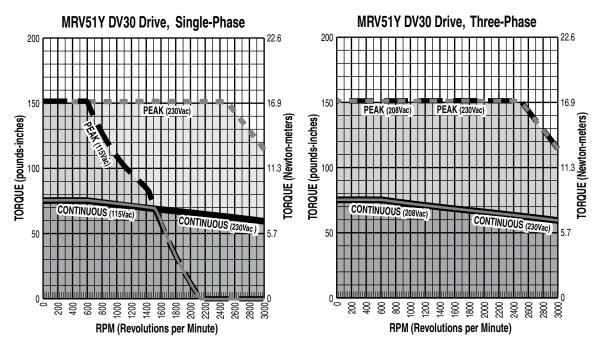
Figure C.12- MRV 51Z DV30 Single-Phase, Three-Phase Drive
