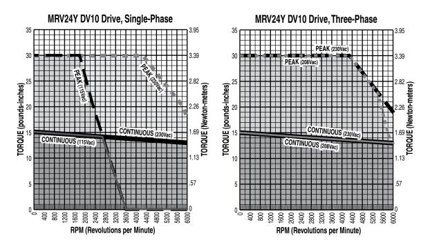
Figure C.5- MRV 24Y DV10 Single-Phase, Three-Phase Drive
