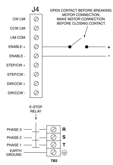
Figure 6.6 - Drive remains powered
