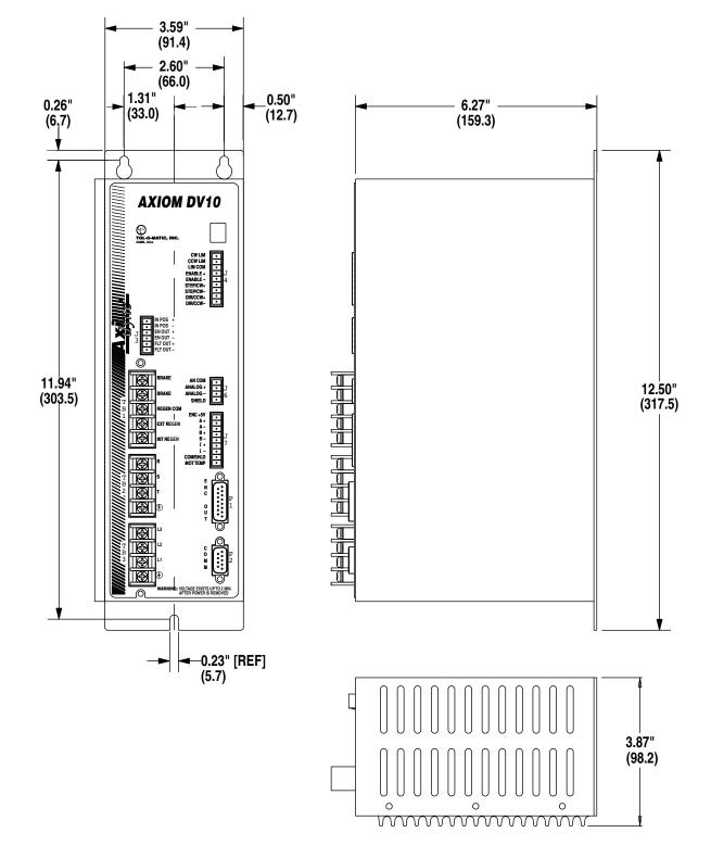
Figure 4.1 - Axiom DV10 Drive Mounting Dimensions
