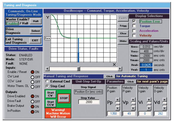
Figure 12.6 Critically Damped Set Command in Position Mode.
