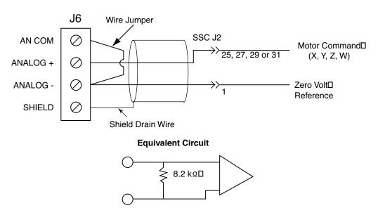
Connection to Tol-O-Matic SSC controller or□ other controller with single-ended output.
