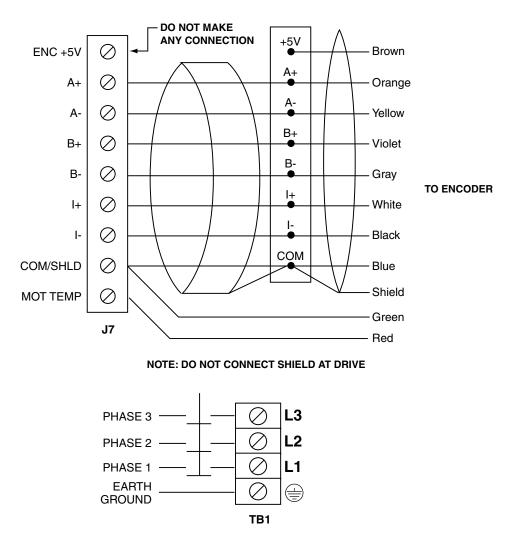
Figure 6.7 - Encoder powered from the motion controller
