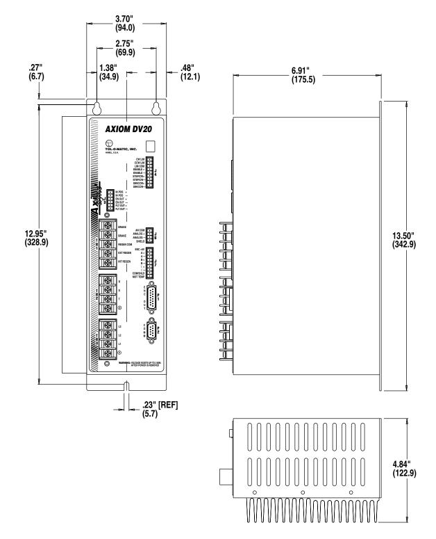
Figure 4.2 - Axiom DV20 and Axiom DV30 Drive Mounting Dimensions
