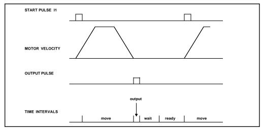
Fig. 9.1 - Motor Velocity and the Associated input/output signals
