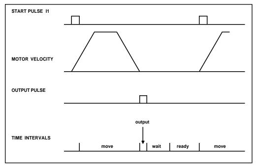
Figure 6.1 - Motor Velocity and the Associated input/output signals
