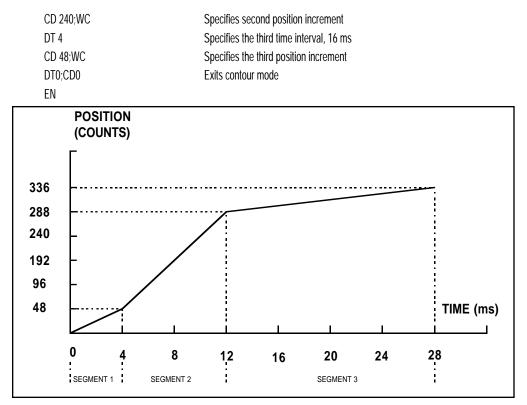
Figure 8.5 - The Required Trajectory
