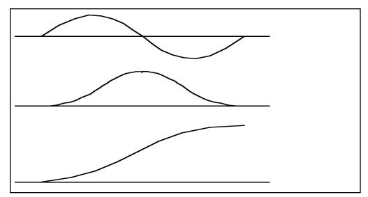
Figure 8.6 - Velocity Profile with Sinusoidal Acceleration
