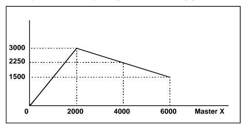
Figure 8.4 - Electronic Cam Example
