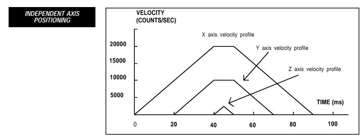
Figure 8.1 - Velocity Profiles of XYZ
