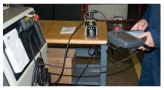
Final system test ensures the feedback device is properly aligned with the GSWA motor poles.
