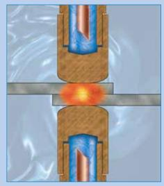
This illustration shows how a weld nugget is formed. The tips of the weld gun are programmed to close rapidly then slow to a 'soft touch' speed as they come in contact with the part for reduced part impact and low expulsion resulting in higher quality welds.
