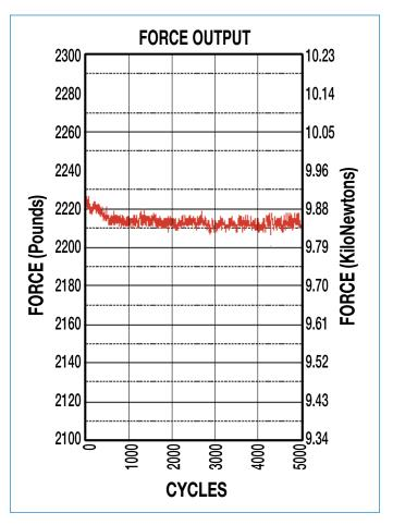
The force output data in this chart is from GSWA actuator run at a fixed current. Each sample is representative of a single "weld cycle." The test was run for 4-1/2 hours.
