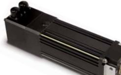
GSWA integrated motor actuator uses an 8 pole, Nd-Fe-B hollow core rotor with skewed stator laminations. This allows the magnet to remain over multiple windings throughout the weld cycle for maximum torque efficiency and consistent force output at any location along the actuator stroke.
