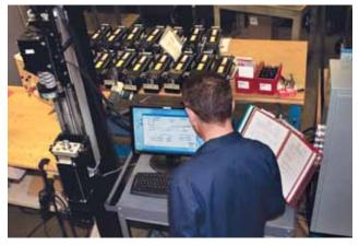
Functional unit testing for 350 cycles quantifies stroke, length, torque under no load, input current vs force standard deviation.
