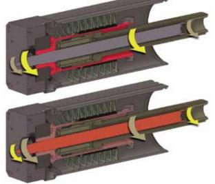
**3.** The nut, mechanically captured by the thrust rod, moves in a linear motion. The bearing and front plate of the GSWA prevents the nut/thrust rod assembly from rotating.
