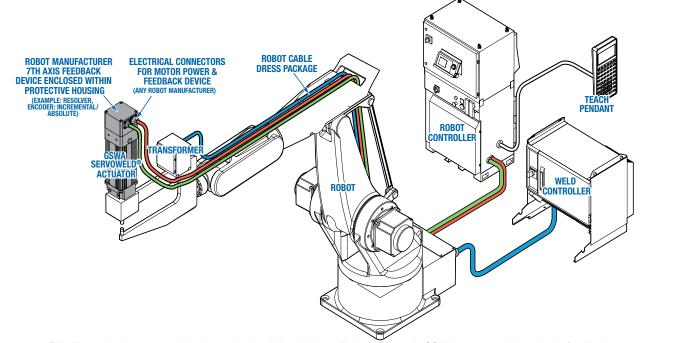
This illustration shows a typical robot carried weld installation utilizing a Tolomatic GSWA actuator with a 7th axis feedback device enclosed within the actuator.
