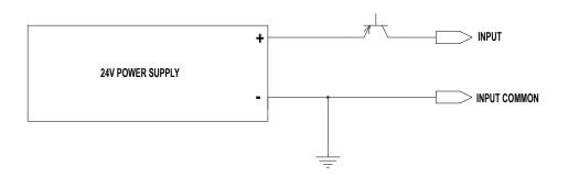
Figure 6-3: Input Source (PNP) Connection
