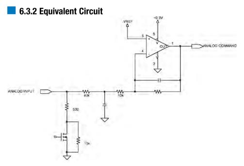
Figure 6-9: Analog Input Equivalent Circuit
