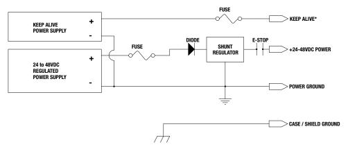
Figure 6-16: Regulated Power Supply with Blocking Diode and Shunt Regulator
