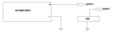
Figure 6-8: Digital Output Sourcing Connection
