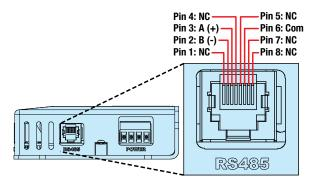
Figure 5-9: ACS 2-Wire RS485 with RJ45 Socket
