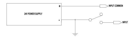
Figure 6-4: Input Sink (switched) Connection
