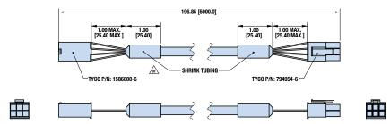
Figure 5-2: Motor Power Cable 3604-1767/1766
