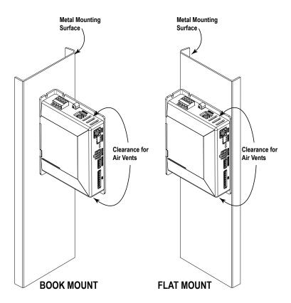
Figure 2-2 Mounting the ACS Drive
