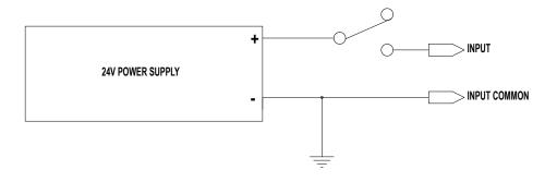
Figure 6-2: Input Source (switched) Connection
