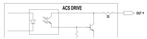
Figure 6-6: Output Circuit
