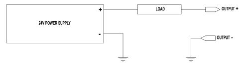
Figure 6-7: Digital Output Sinking Connection
