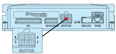
Figure 5-1: Motor Power Connection on ACS Drive
