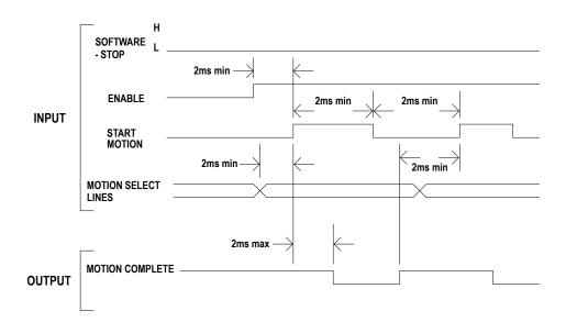
Figure 7-4 Absolute & Incremental Move Timing
