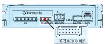
Figure 5-3: Encoder Connection on ACS Drive
