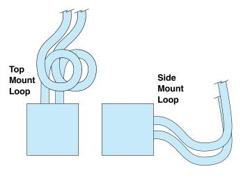
Figure 5-12 Cable Routing for Top and Side Facing Connectors
