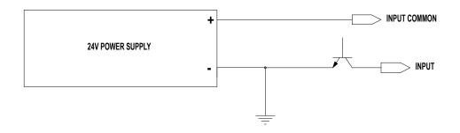
Figure 6-5: Input Sink (NPN) Connection
