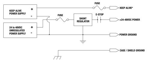
Figure 6-14: Unregulated Power Supply Configuration with Shunt Regulator
