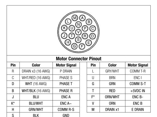
**Table A-3: Motor Connector pinout**
