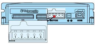
Figure 5-2: Motor Power Connection on ACS Servo Drive (repeated for reference)
