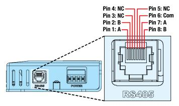
Figure 5-10: ACS 2-Wire RS485 with RJ45 Socket
