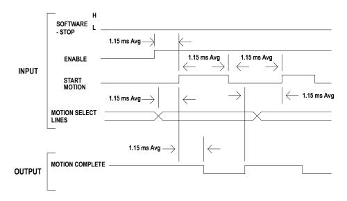
Figure 7-4 Absolute & Incremental Move Timing
