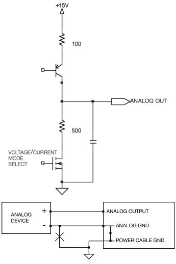
Figure 6-10: Analog Output Equivalent Circuit
