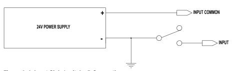
Figure 6-4: Input Sink (switched) Connection
