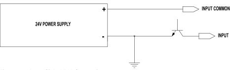
Figure 6-5: Input Sink (NPN) Connection
