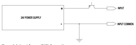
Figure 6-3: Input Source (PNP) Connection
