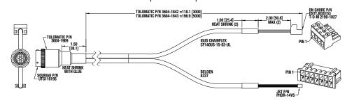
Figure 5-1: Motor Power/Encoder Cable 3604-1842, 3604-1843, 3604-1943
