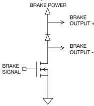
Figure 6-11: Brake Output Equivalent Circuit
