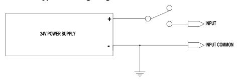
Figure 6-2: Input Source (switched) Connection
