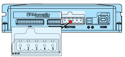
Figure 5-2: Motor Power Connection on ACS Servo Drive
