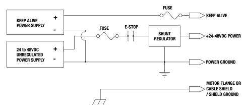
Figure 6-13: Power Supply Configuration with Shunt Regulator
