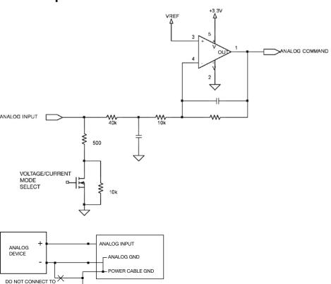
Figure 6-9: Analog Input Equivalent Circuit
