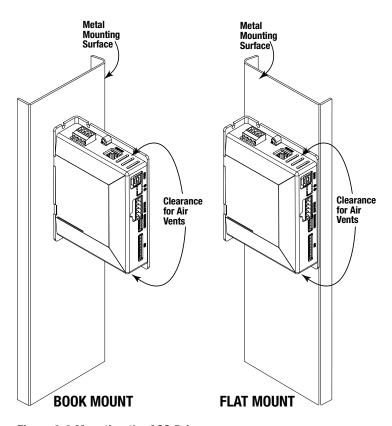
Figure 2-2 Mounting the ACS Drive
