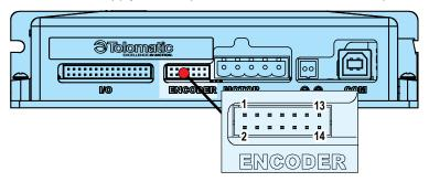
Figure 5-3: Encoder Connection on ACS Drive
