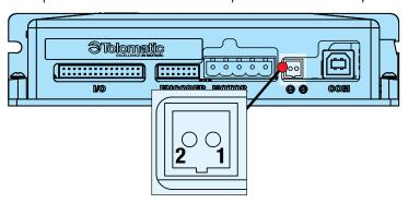
Figure 5-7: Brake Connection
