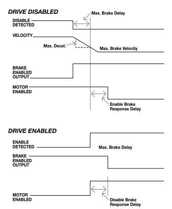
Figure 7-5 Brake Subsystem Timing
