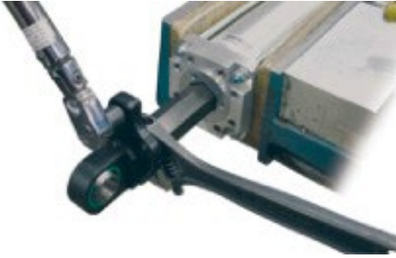
Figure 4.4: For Hex rod, hold thrust rod stationary using a wrench on the flat of the rod when attaching accessories, linkages or load to the actuator. Use a torque wrench to tighten the interfacing rod end to the actuator threaded connection point. Torque values provided in Table 4.1
