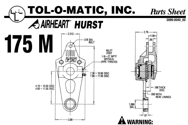
MOUNTING: Proper Bracketry is essential to insure against brake failure and should be fabricated only by an experienced professional. Only use fluid taken from an unopened container or one which has been tightly closed. Brake fluid will absorb water from the atmosphere which will cause fluid boiling at much lower temperatures and will result in loss of brakes.
