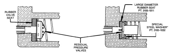
\*SPECIAL STEEL WASHER IS NECESSARY TO INSTALL VALVE IN 3/4" DIAMETER STRAIGHT BORE MASTER CYLINDER — (NO STEP DIAMETER IN BORE). EARLY PRODUCTION MASTER CYLINDER (WITH STEPPED BORE) REQUIRES SMALLER DIAMETER RUBBER SEAT — (PT. 3110 1007). STEEL WASHER CANNOT BE USED WITH STEPPED BORE.
