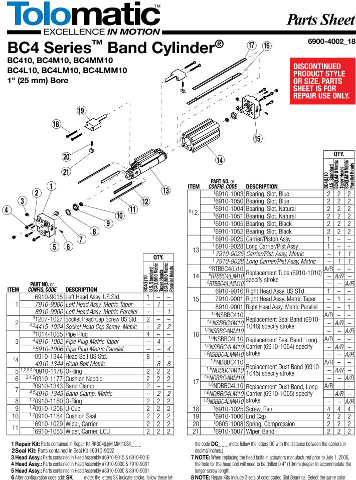
6 After configuration code add: **SK**\_\_\_ (note: the letters SK indicate stroke, follow these letters with the stroke length in decimal inches.) If the actuator has the dual carrier option add
