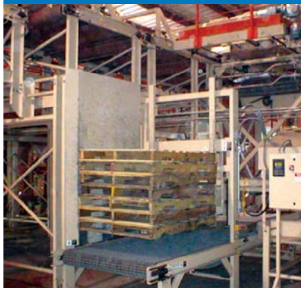
Slip sheet placement on pallets for palletizing.
