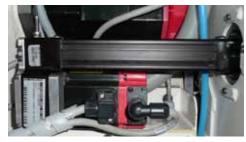
Tolomatic's RSM actuator features a reverseparallel motor drive with the motor mounted along side theactuator, driving the screw through a toothed belt and pulley assembly. The compact actuator series is designed for high-performance thrust from 70 to 7,000 pounds, accuracy and durability.
