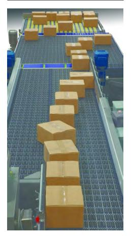
Tolomatic ERD electric actuators are used to organize pallet layers in the Intralox ARB™ alignment conveyor system.
