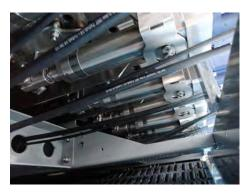
The low-maintenance features of the Tolomatic ERD actuators are important in this application due to the tight mounting quarters.
