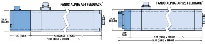
\*Shown fully assembled with customer supplied feedback
