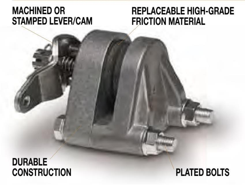
Tolomatic manufactures a broad range of mechanical brakes in these series: ME10, ME20, ME220 and MB3. Designed for use in areas that do not have access to other types of power, these single acting calipers feature replaceable, high-grade friction material, aluminum or cast iron construction (depending on model) and zinc plated bolts. (See pages 56 to 65)
